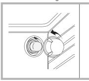
Remove the light bulb and replace it with a similar one: Wattage 25 W, cap E 14.
